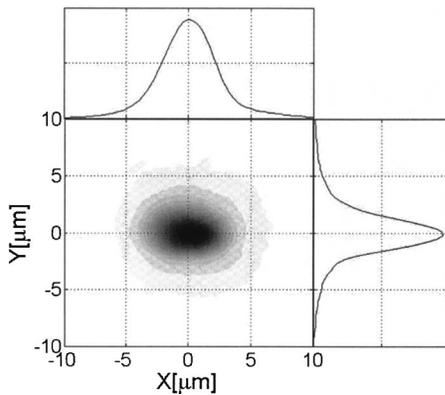
Fig. 1. Intensity profile of the fundamental mode of the waveguide at  $1.55 \mu\text{m}$ .
