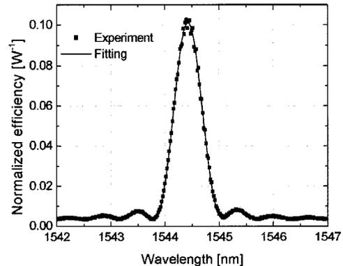
Fig. 2. Bulk second-harmonic generation efficiency versus wavelength (experimental conditions:  $25 \text{ mm}$  long sample,  $21 \mu\text{m}$  poling period,  $107 \mu\text{m}$  beam radius).
