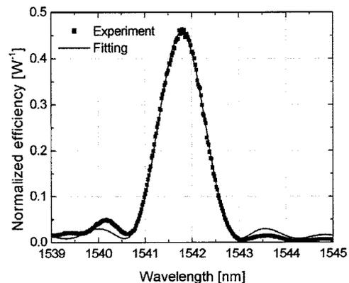
Fig. 3. Waveguide second-harmonic generation efficiency versus wavelength.
