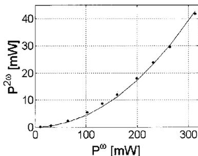
Fig. 4. Dots, second-harmonic output power versus input pump power as measured in room-temperature operating conditions. Solid curve, expected curve from low pump-depletion characterization.
